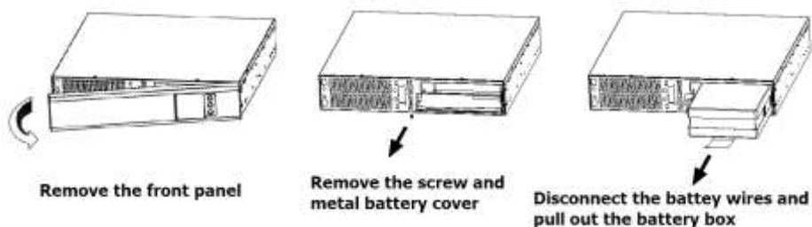
Fig.8 Replacing battery
